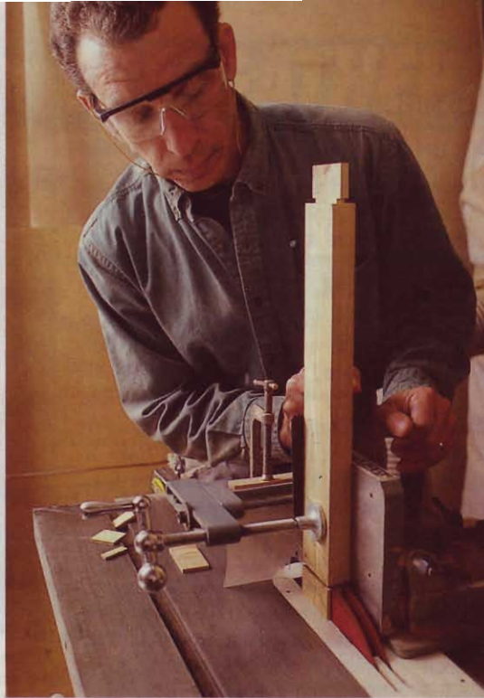
John Thomson, production manager, cuts tenons on the shop-built tenoner, a benchtop tablesaw fitted with a split dado set.
